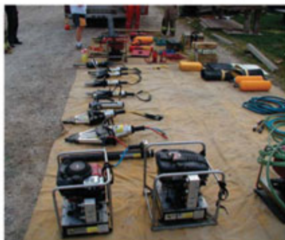
Staging tools at an MVC helps to speed-up the rescue operation. Laying tools out in a particular, sequential order helps us to quickly find the one we're looking for when it's needed.
